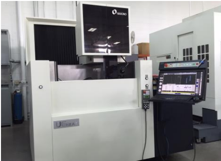
Makino U6 H.E.A.T. Wire EDM with drop tank and 25.5 x 17.7 x 16.5 (Z) travels
