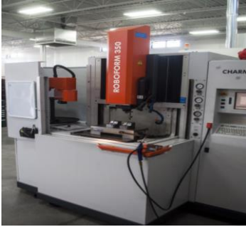
Charmilles Roboform 350 CNC EDM w/ 3R macro combi tooling 32 station tool changer. (14 x 10 x 14 working envelope)
